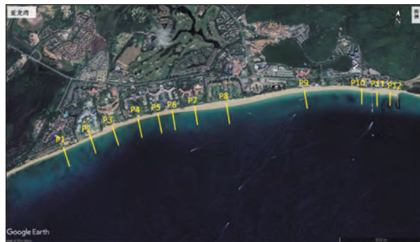
图8 12个海滩测量断面布设图 Fig.8 Layout of 12 beach surveying profiles
